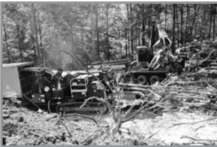
Wood not suitable for logs is chipped and used for fuel by a hybrid power plant.
